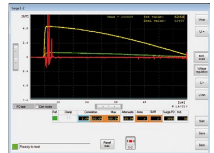
Surge voltage pulse with 150 ns, rise time, and PD-effects
