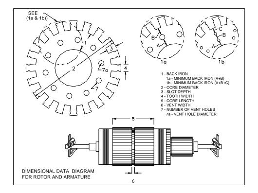
5. Click on *Automatic Core Loss* Test to proceed with the test. The computer calculates the test voltage required to produce the desired flux density in the back iron and recommends the appropriate output tap. It will then prompt the operator to connect the output power and voltmeter cables.
