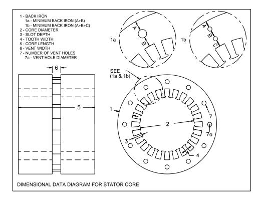
Click on Automatic Core Loss Test to proceed with the test. The computer calculates the test voltage required to produce the desired flux density in the back iron and recommends the appropriate output tap. It will then prompt the operator to connect the output power and voltmeter cables.
