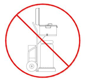
DO NOT OPERATE THE TEST SET WITHOUT REMOVING HIGH-VOLTAGE TRANSFORMER FROM THE CART.
